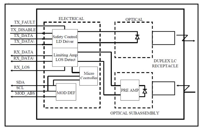
**Transmitter Section-** The DFB laser driver accept differential input data and provide bias and modulation currents for driving a laser. An automatic power-control (APC) feedback loop is incorporated to maintain a constant average optical power.1550nm in an eye safe optical subassembly (OSA) mates to the fiber cable.
